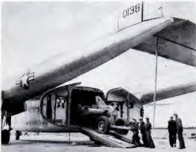
Big scraper is loaded aboard a flying boxcar at Seven Islands for a flying journey to the railroad builders far up the line
